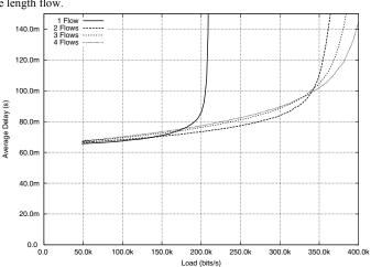
Fig. 9. Cross configuration five hop average end-to-end delay. When the throughput is low, more flows produces a larger delay due to the increase probability of collisions.
