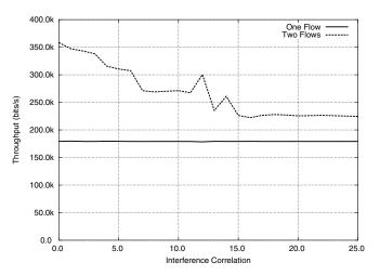
Fig. 11. Maximum aggregate throughput versus interference correlation. The throughput decreases with the correlation.
