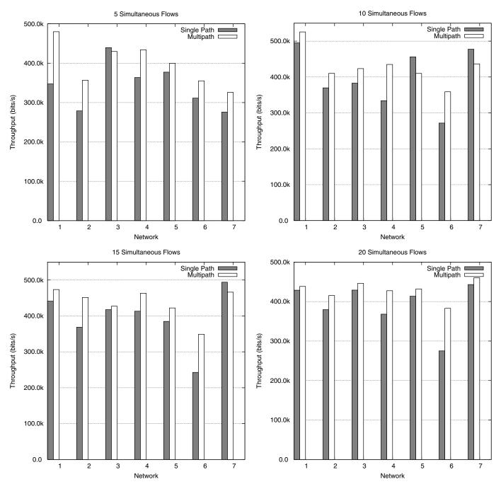
Fig. 13. Grid network aggregate throughput. This shows that using multipath routing can improve the aggregate throughput of grid networks in the majority of cases. It appears that multipath performance depends strongly on the traffic pattern, as all of these scenarios have the same topology, but use different paths.
