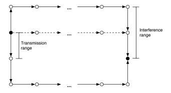
Fig. 5. Load balancing in a large grid network. The paths are forced away from the shortest path, shown with the dashed line, to ensure that the two paths are out of interference range of each other.
