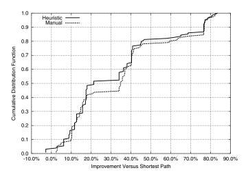
Fig. 12. Cumulative distribution function of the throughput improvement. The performance of the manual and the heuristic schemes is very similar.
