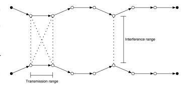
Fig. 6. Two paths with an interference correlation of five.
