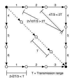
Fig. 4. The rate-limited transmission schedule for a simple 4×4 grid topology.
