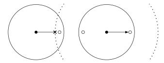
Fig. 1. Interfering transmissions in a chain of nodes. The transmission at the left hand side is unsuccessful due to the interference from the right hand transmission.
