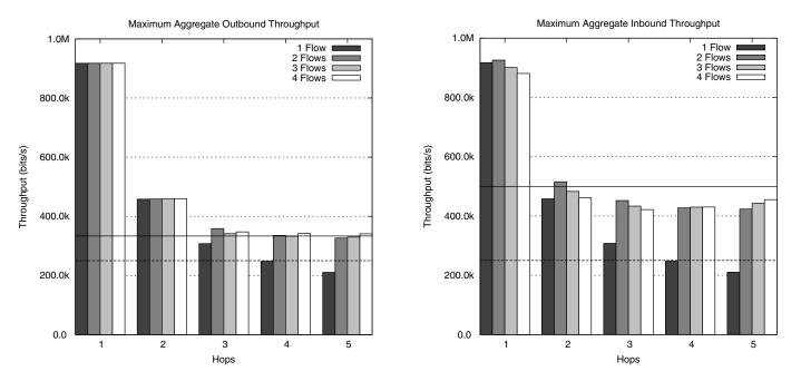
Fig. 8. Cross configuration maximum aggregate throughput. The solid lines mark the analytical multipath throughput for an infinite length chain with rate limiting, and the dashed lines indicate the analytical throughput for a single infinite length flow.
